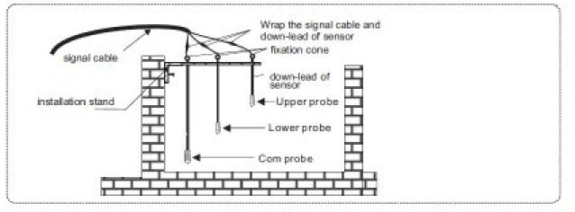
In event of high risk of electric storms (lightning) or when liquid medium in well or tank or sump is very dirty it is recommended float switch is used.
