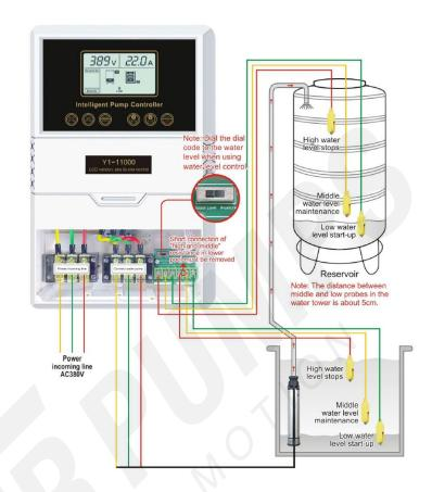
Note: Avoid Signal Line Short Circuits: Ensure no entanglement with power or pump lines, and steer clear of areas with strong interference from electrical appliances like transformers or signal towers.
