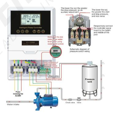
Note: Avoid Signal Line Short Circuits: Ensure no entanglement with power or pump lines, and steer clear of areas with strong interference from electrical appliances like transformers or signal towers.
