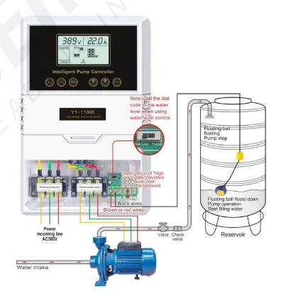
Note: Avoid Signal Line Short Circuits: Ensure no entanglement with power or pump lines, and steer clear of areas with strong interference from electrical appliances like transformers or signal towers.
